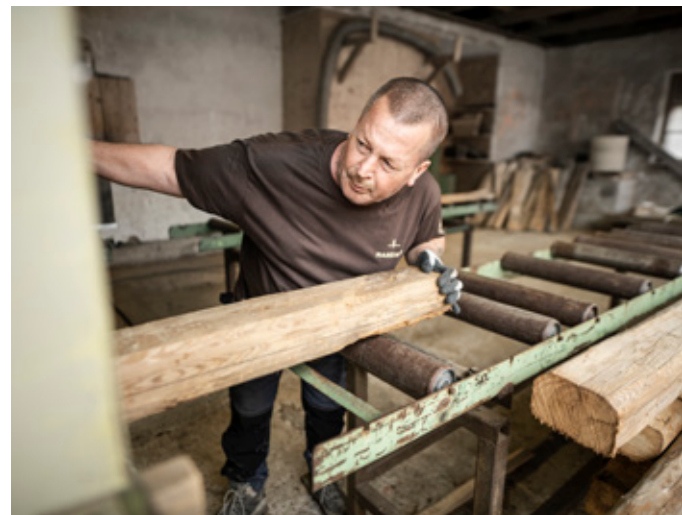
Franz (above) and Jürgen (right) run the old wood hairdressing salon: So much brushing happens here that it is a true splendor. Jürgen loads the brushing machine, mostly with old beams and rafters. After they are run through, Franz goes over them again manually.
